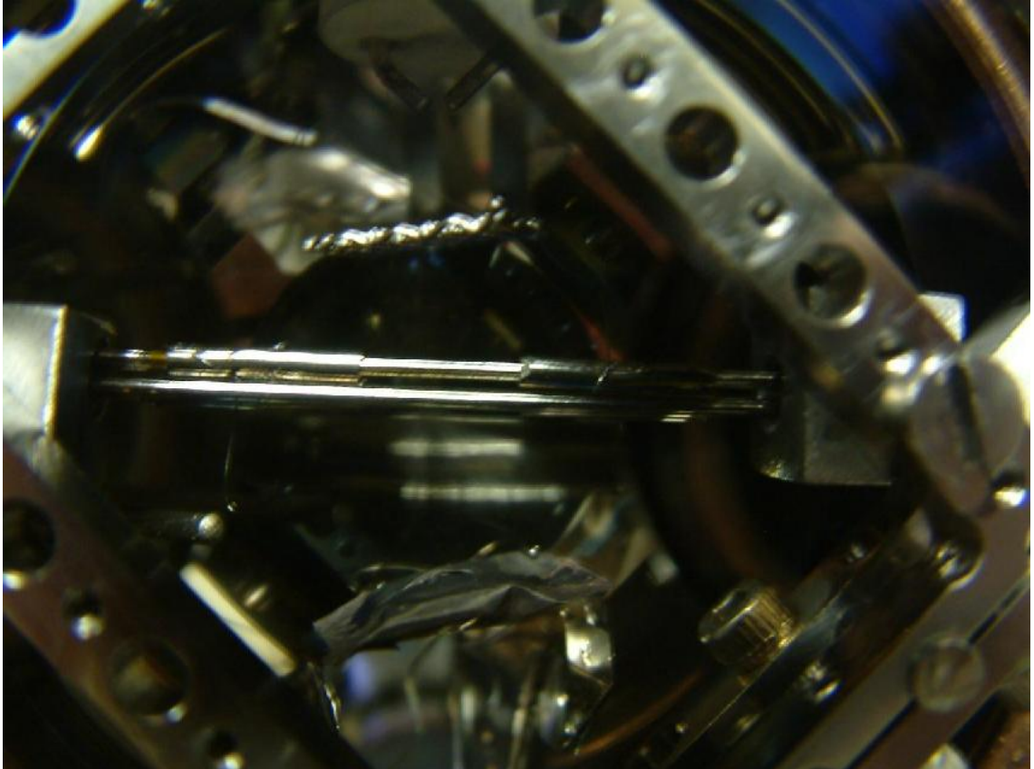
Figure 15: The first functional ion trap built for this experiment. It has a trap radius r_0 = 0.89 mm, length l = 8 mm and operates at a frequency \Omega = 2\pi \cdot 6.6 MHz. Above the trap is a tungsten filament used for electron-impact ionization. Below the trap is a small resistively heated barium oven. Cooling and photoionization light passes through the trap at 45^\circ to its axis.
