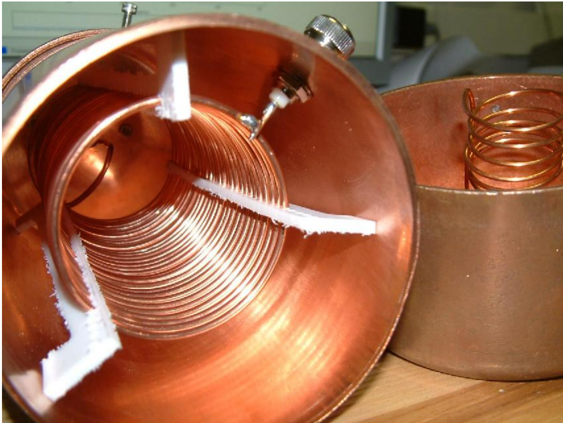
Figure 16: Photograph of the quarter-wave coaxial resonator used to produce high voltage rf. It had a resonance quality factor Q \approx 100 and was capable of outputting >200 V at 6.6 MHz. Rf was coupled into the low voltage end using a small loop antenna (pictured right) whose position was adjusted until coupling into the resonator was maximized. The weight of the helix is supported by three teflon ‘combs.’ Teflon is used for this purpose because of its low rf loss-tangent.
